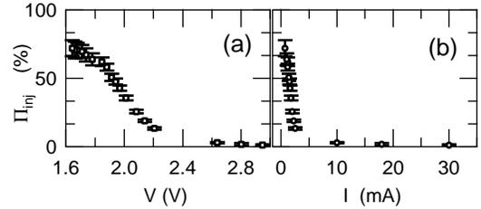
FIG. 1: The degree of injected spin polarization measured at 4.6 K as a function of the applied bias voltage (a) and the current (b) from Ref. 4.
