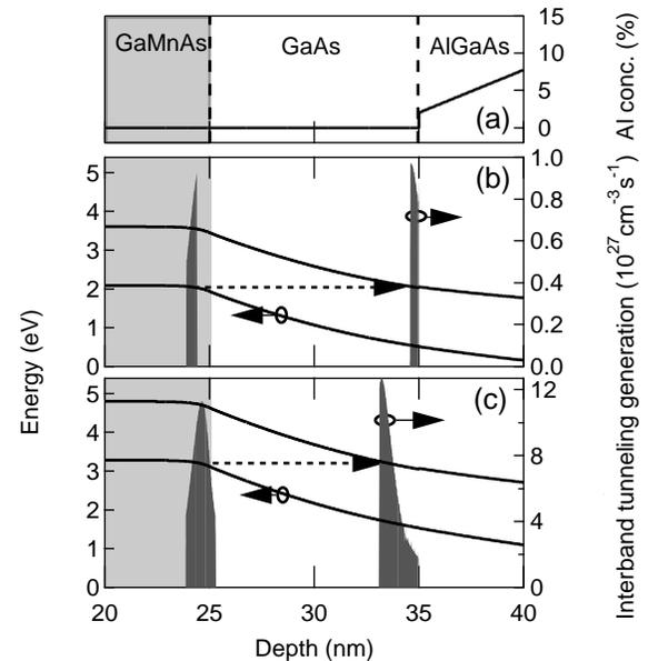
FIG. 3: The Al concentration (solid line) (a), the band diagram (solid lines) and the carrier generation (filled) due to interband tunneling (dotted line) as a function of the depth near the (Ga,Mn)As/GaAs tunnel diode at 1.8 V (b) and 3 V (c). The grey-coloured area represents the (Ga,Mn)As injector. The dotted arrows indicate the tunneling of valence electrons from (Ga,Mn)As to GaAs.
