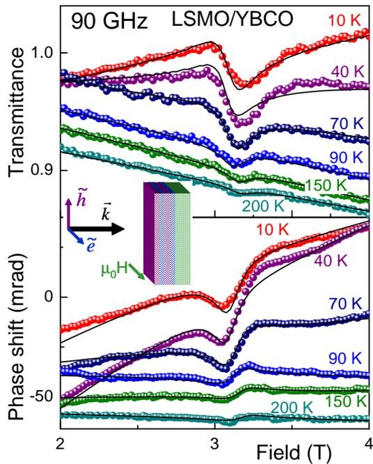
FIG. 2: Magnetic field-dependence of the transmittance (upper panel) and the phase-shift (lower panel) of the LSMO/YBCO superlattices at  $\nu = 90$  GHz and for different temperatures. Symbols - experiment, lines - fits to the Lorentz-like form of the ferromagnetic resonance close to 3.1 T. The inset shows the geometry of the experiment.
