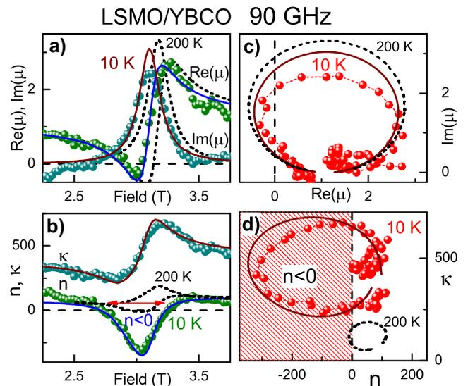
FIG. 3: Magnetic permeability of LSMO/YBCO superlattices at  $T = 10$  K as function of magnetic field (a) and replotted in the complex-plane (c). The complex refractive index as field-dependence (b) and in the complex plane (d). The shaded area corresponds to the region with negative real part of refractive index. The results for  $T = 200$  K are given for comparison. In all frames the symbols correspond to experimental data, lines represent the Lorentz model for the FMR line.
