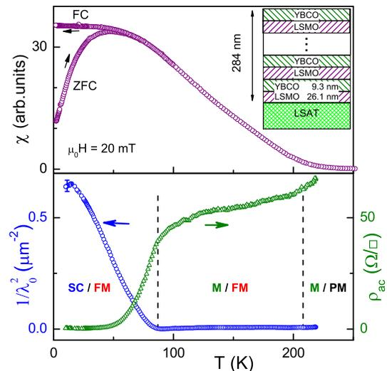
FIG. 1: Upper panel: Magnetic susceptibility of the LSMO/YBCO superlattice measured in the field-cooling (FC) and zero-field-cooling regime (ZFC). The inset shows schematically the composition of the sample.
