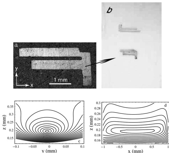
FIG. 2: (a) Foil atom chip. (b) Photograph of two FePt structures with slightly different dimensions glued on an aluminum mirror. (c)  $y$ - $z$  and (d)  $x$ - $z$  plots of the calculated magnetic stray field for the lower structure in (b). Shown are contours of equal magnitude of magnetic field  $B$  (i.e. equipotential lines), with a spacing of 6 G between the contours, in planes containing the trap minimum. The chip surface is at  $z=0.2$  mm.
