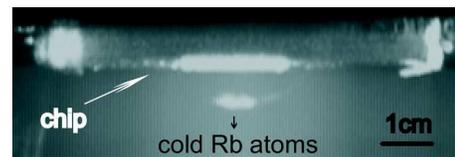
FIG. 3: Fluorescence image of a cloud of cold  $^{87}\text{Rb}$  atoms under the mirror. Mirror magneto-optical trap, using the stray field of the structure, at about 2 mm below the lower "F" shown in Fig. 2b.
