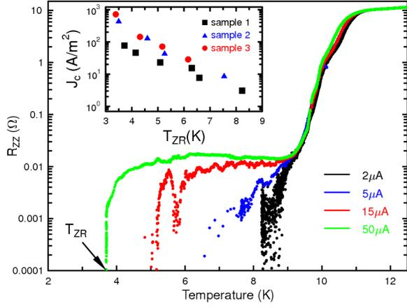
FIG. 1: (Colour online) Temperature dependence of interlayer resistance in zero applied magnetic field, for a range of currents. Inset: critical current density for the onset of dissipation,  $J_c$ , as a function of  $T_{ZR}$ , the temperature at which the resistance becomes zero.
