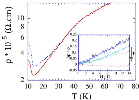
**Fig. 5.** Temperature profile of the chain axis microwave resistivity in zero (full) and 14 Tesla (dotted) magnetic field values. Inset: relative magnetoresistance measured at 14, 16, 18 and 80 K. The right arrow indicates the temperature variation.
