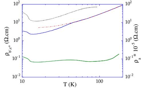
**Fig. 1.** Microwave resistivity of  $(\text{TMTSF})_2\text{PF}_6$  as a function of temperature along  $\mathbf{a}$  (full),  $\mathbf{b}'$  (dashed) and  $\mathbf{c}^*$  (dotted) axes. The dashed-dotted line mimics the behavior of the dc resistivity along the chain axis.
