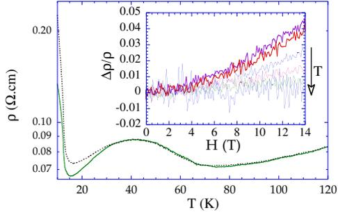
**Fig. 2.** Microwave resistivity along  $\mathbf{b}'$ , in zero (full) and 14 Tesla (dotted) magnetic field values. Inset: relative magnetoresistivity measured at 16, 18, 20, 25, 35 and 80 K. The right arrow indicates the temperature variation.
