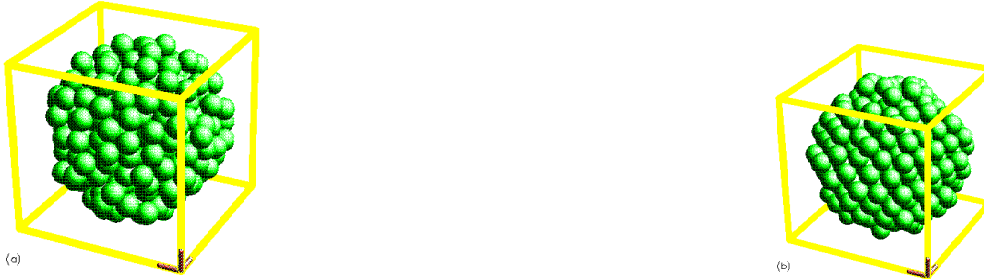
Figure 2. An example of typical clusters obtained after 2000 timesteps for a) A = 0.05 b) A = 0.5 . Note the crystalline-like ordering in the second case
