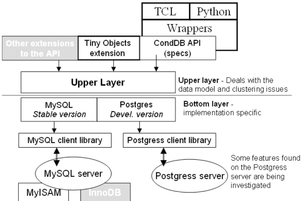
Figure 2: System software layout.
