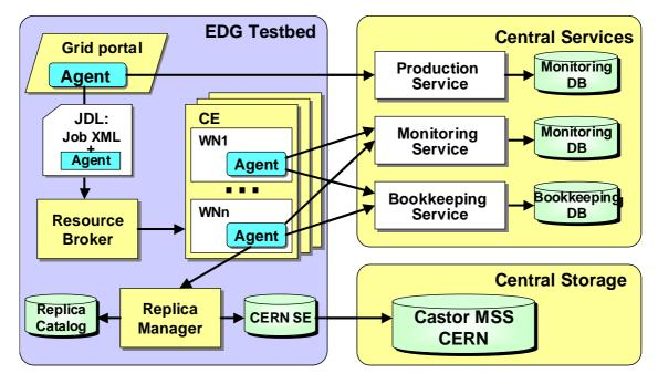
Figure 5: Running DIRAC jobs on the DataGRID
