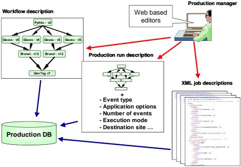
Figure 2: Definition of the production tasks
