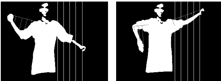
Figure 5: Image Processing Results . Left: Locating outermost tip. Right: Finding the elbow and wrist joints.
