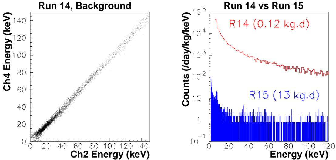
**FIGURE 1.** Left, pulses, as seen by both tungsten films on a common crystal, before removal of source of stress on crystal. All pulses are found to be coincident and to be of same energy within the resolution of the detector, and thus originate within the absorber. The agreement between the two channels is also a check of the consistency of the methods used. Right, typical energy spectra before and after modifying crystal mounting.
