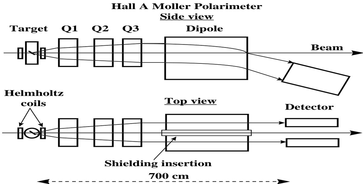
Fig. 1. Hall A Møller polarimeter set-up
