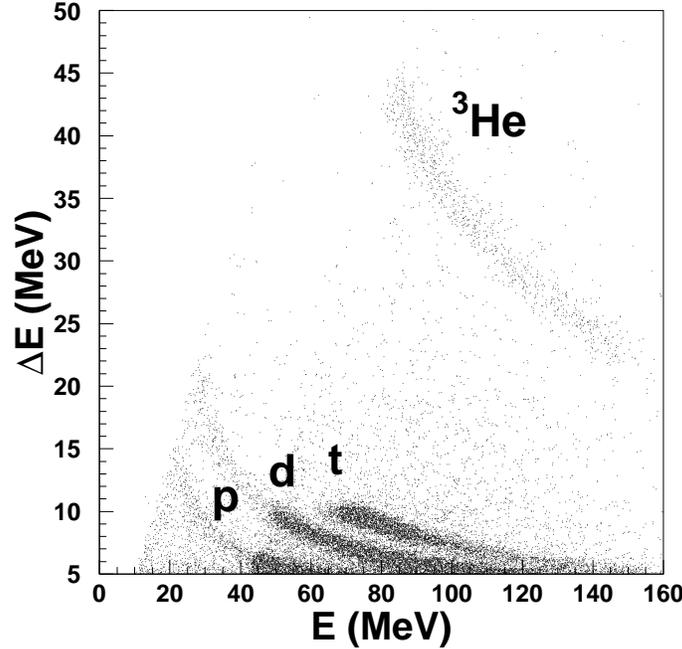
Figure 3. Energy loss in the Quirl as function of the total energy deposited in all detectors. The bands visible are due to detected protons, deuterons, tritons and  ${}^3\text{He}$ .
