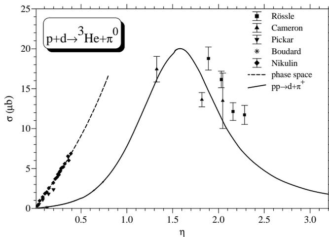
Figure 1. Excitation function for the indicated reaction. Data are shown as symbols with error bars and are from Ref.'s [8–10,7,11]. The result of the Germond-Wilkin model is shown as dashed curve, and the  $pp \rightarrow d\pi^+$  reaction divided by 160 as solid curve.
