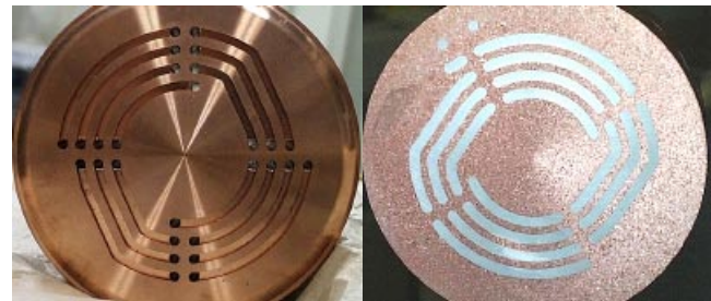
Fig. 2a: Groove processing Fig. 2b: Filling with silver powder coated wax for the water-cooling channel.
