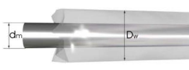
Fig. 3. Sketch of the glass covered wire. The core has a diameter  $d_m$ , whilst the total diameter of the micro wire, i.e. core and the glass coating, is  $D_w$ .
