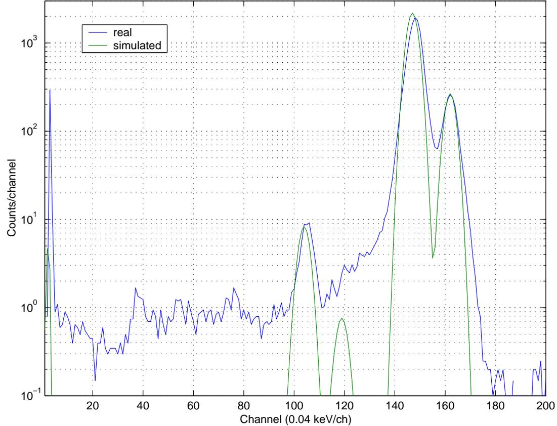
**Figure 6.** A simulated  $^{55}\text{Fe}$  calibration spectrum (green line) in comparison to a measured spectrum (blue line). The underground apparent between channel 10 and 140 is due to non-linearities in the detector response function (see Fig. 5).
