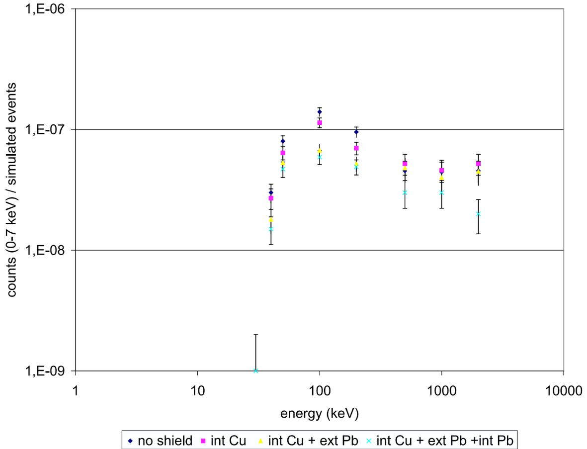
**Figure 7.** Response of the pn-CCD to external  $\gamma$ -ray background. The energy of the incident  $\gamma$ -ray photon versus the number of detected counts in the 0–7 keV is shown relative to the number of simulated events for different configurations of the shield. Results are shown for an unshielded detector, the copper box (int Cu), an additional Pb shield outside the vessel (ext Pb), and an additional Pb shield inside the vessel being installed (int Pb).
