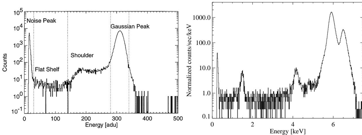
**Figure 5.** Left: Spectral energy response of an XMM-Newton EPIC pn-CCD similar to the one in use for CAST, for an incident monochromatic photon energy of 1.4 keV.<sup>13</sup> Right: Spectrum of an  $^{55}\text{Fe}$  calibration source measured with the CAST detector. The Al-K line apparent at 1.5 keV originates from an aluminum filter installed in front of the  $^{55}\text{Fe}$  calibration source.
