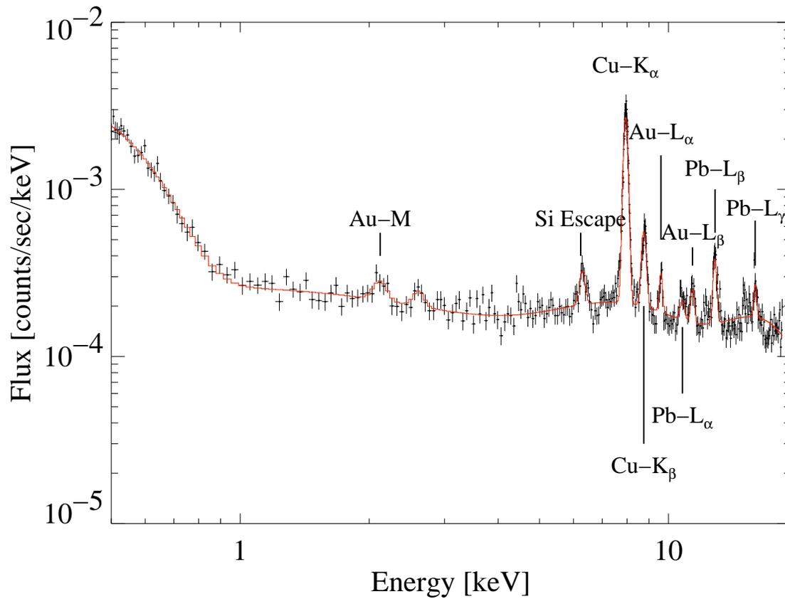
**Figure 4.** Background spectrum observed with the pn-CCD detector in the CAST environment. The overall background is composed of contributions from fluorescent emission of Pb, Cu, and Au on top of a continuum spectrum. The peak at energies  $E < 1$  keV corresponds to low energy noise. The X-rays from axion to photon conversion are expected to be thermally distributed between 1.0 keV and 8 keV.
