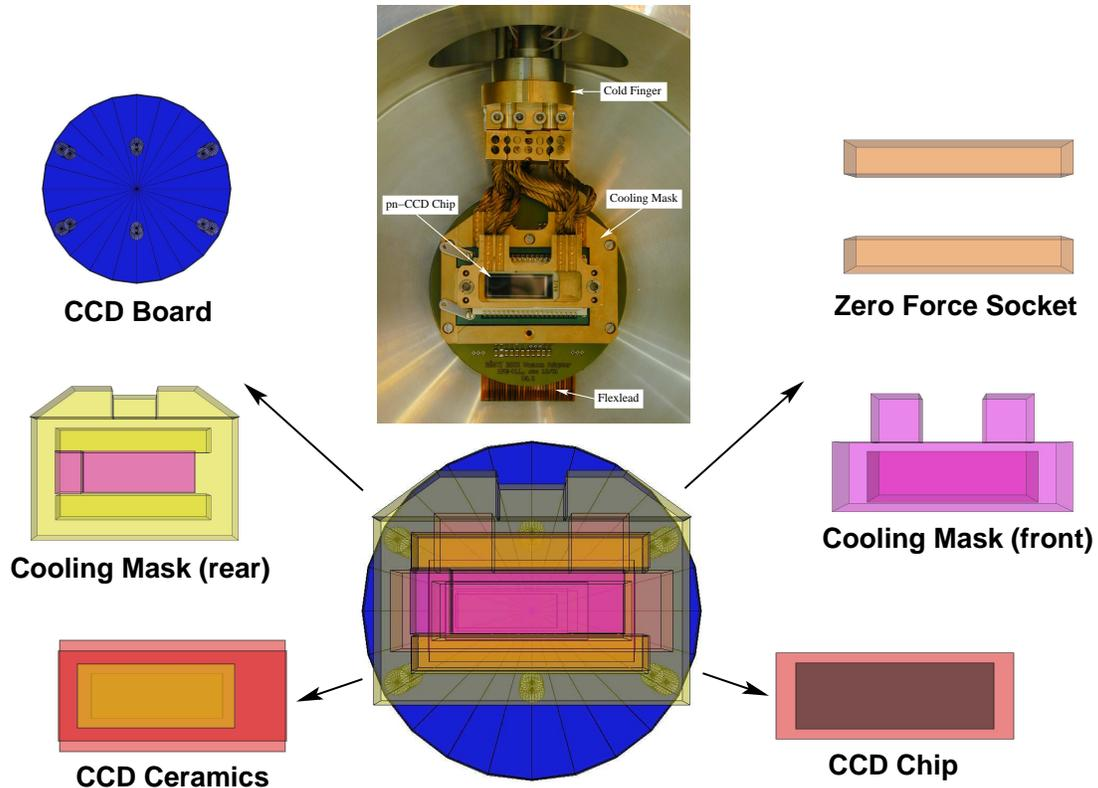
**Figure 2.** Top Center: The pn-CCD chip (black part in the center) with the gold plated cooling mask which is connected to a cold finger of a Stirling cooler device. The individual detector components as modeled in GEANT4 are shown below and to the left and right. Due to the limited time for R&D these components were tested for their natural radioactivity in the Canafranc underground laboratory,<sup>10</sup> but not built from selected and radio-pure materials.
