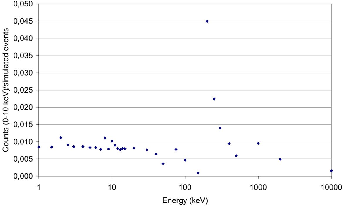
**Figure 8.** Response of the pn-CCD to the neutron background.
