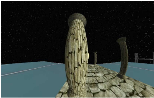
FIG. 4: Screenshot from Real Time Relativity showing relativistic aberration. The camera is moving towards the center of the column with v = 0.9682c , so that \gamma = 4 . The Doppler and headlight effects are off.
