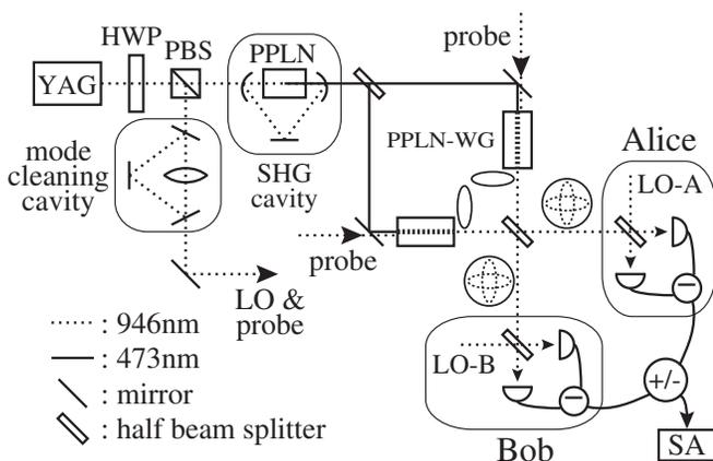
Fig. 1: The experimental setup for generation of broadband EPR beams. HWP: half wave plate, PBS: polarization beam splitter, PPLN-WG: periodically-poled lithium niobate waveguide, LO: local oscillator, SA: spectrum analyzer. The ellipses indicate the squeezed quadratures of each beam.
