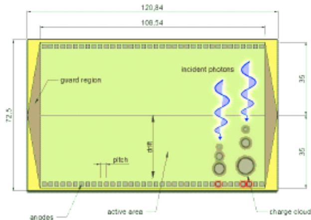
Figure 1. *LOFT* Silicon Drift Detector scheme
