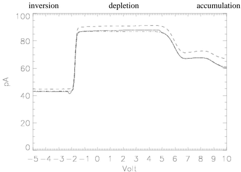
Figure 10. I-V curve for GD#3 measured at INFN-Trieste before and after proton irradiation (*dotted* line=4 days after irradiation, *dotted-dashed* line=11 days after irradiation)
