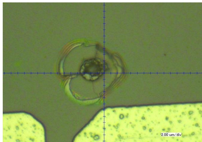
Figure 15. Microscope view of a crater produced in the voltage divider area by a debris impact
