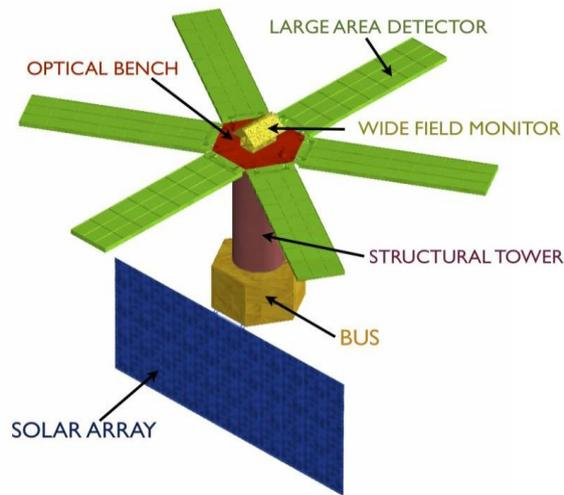
Figure 2. LOFT conceptual scheme (courtesy of ISDC)
