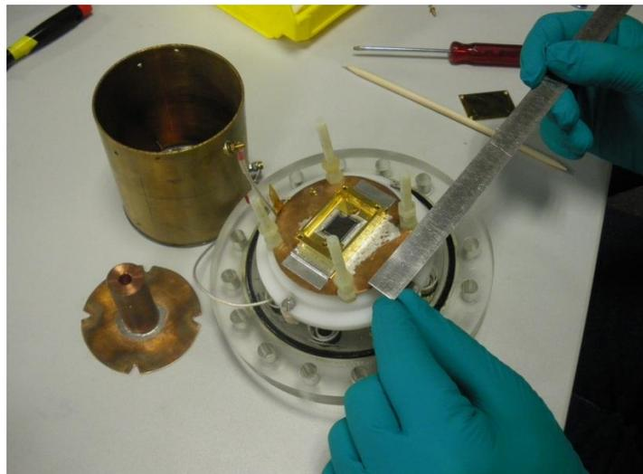
Figure 16. A 6x6 array of GSFC micro-calorimeters mounted in the small test chamber at MPIK for debris impact test
