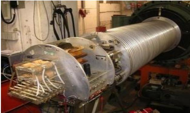
Figure 12. Accelerating coils
