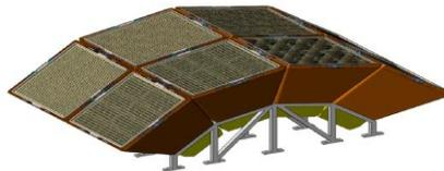
Figure 4. WFM: 8 co-aligned cameras (4 units)
