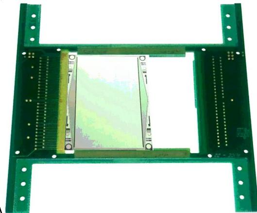
Figure 8. SDD+PCB prototype for soft proton test
