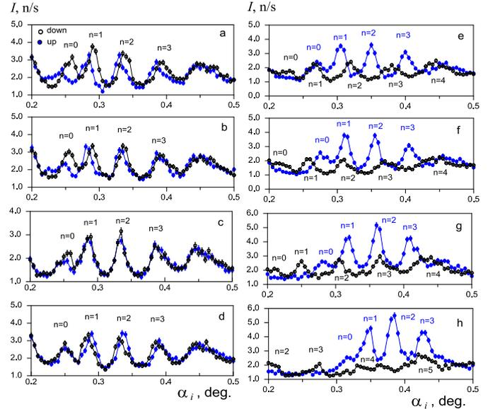
Fig. 8. Neutron microbeam intensity for spin up (closed symbols) and spin down (open symbols) vs. the grazing angle of the incident beam in the applied magnetic field: (a) 18 Oe; (b) 194 Oe; (c) 395 Oe; (d) 595 Oe; (e) 2010 Oe; (f) 3020 Oe; (g) 4007 Oe and (h) 11400 Oe.
