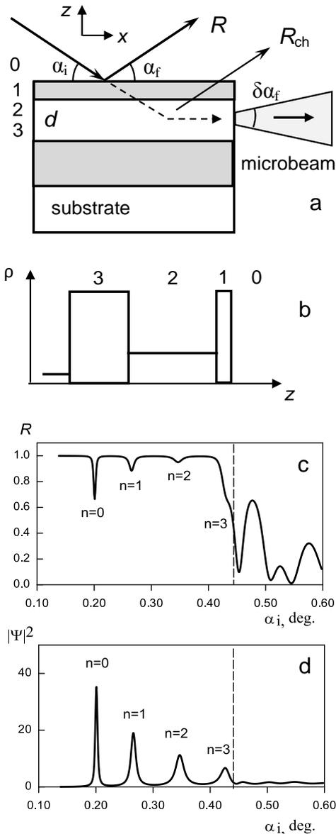
Fig. 3. Planar waveguide: (a) geometry; (b) SLD; (c) reflectivity; (d) neutron wavefunction density.
