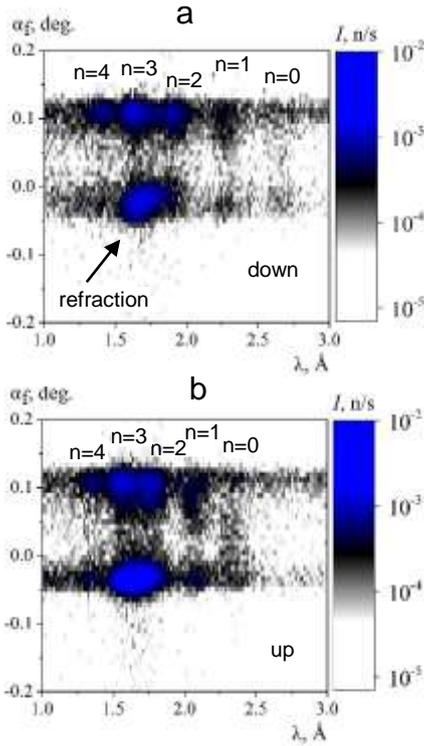
Fig. 12. The neutron intensity at the grazing angle of the incident beam  $0.133^\circ$  vs. the neutron wavelength and the grazing angle of the scattered beam for spin down (a) and up (b). The applied field is 1500 Oe.
