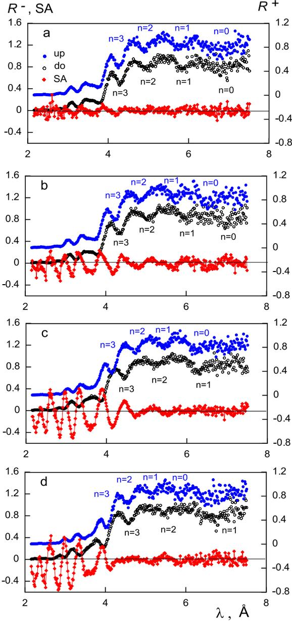
Fig. 15. The reflectivities for spin up (closed circles) and down (open circles) and the spin asymmetry (rhombi) are presented vs. neutron wavelength for the different applied magnetic field: (a) 600 Oe; (b) 1114 Oe; (c) 3030 Oe and (d) 7001 Oe. The grazing angle of the incident beam is  $0.397^\circ$ .
