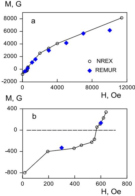
Fig. 10. The magnetization extracted from splitting of the microbeam intensity peaks  $n=0$  vs. the applied magnetic field: (a) total interval; (b) zoom around the coercive field. Open and closed symbols correspond to the results obtained on NREX and REMUR reflectometers respectively.
