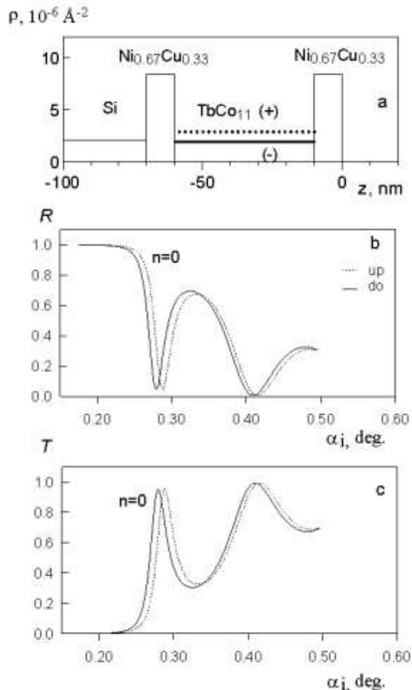
Fig. 16. Calculations for the interference filter  $\text{Ni}_{0.67}\text{Cu}_{0.33}$  (10nm)/ $\text{TbCo}_{11}$  (50)/ $\text{Ni}_{0.67}\text{Cu}_{0.33}$  (10)//Si (substrate) for the neutron wavelength 4.26 Å. (a) SLD vs. coordinate  $z$  perpendicular to the sample surface. (b) Reflectivity for spin up (dashed line) and spin down (solid line). (c) Transmission coefficient for spin up (dashed line) and spin down (solid line).
