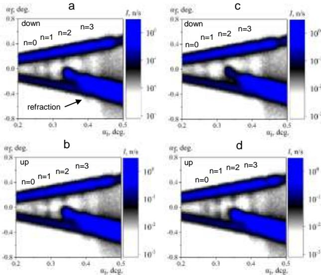
Fig. 7. Neutron intensity vs. the grazing angle of the incident and the scattered beams for the applied field: (a) 595 Oe for spin down; (b) 595 Oe for spin up; (c) 2010 Oe for spin down; (d) 2010 Oe for spin up. The neutron wavelength is 4.26 Å.
