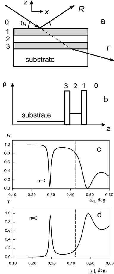
Fig. 1. Interference filter: (a) geometry; (b) SLD; (c) reflectivity; (d) transmission coefficient.
