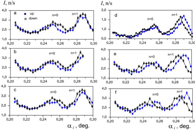
Fig. 9. Neutron microbeam intensity for spin up (closed symbols) and spin down (open symbols) vs. the grazing angle of the incident beam around coercive field: (a) 451 Oe; (b) 530 Oe; (c) 551 Oe; (d) 570 Oe, slit1=0.25 mm; (e) 620 Oe; (f) 640 Oe.
