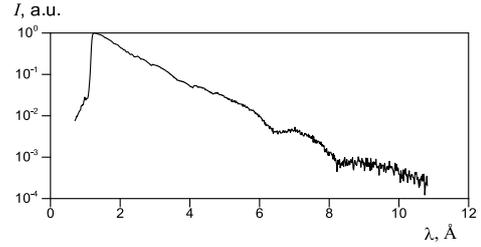
Fig. 11. The neutron spectrum at the REMUR reflectometer from the combined (thermal and cryogenic) moderator of the pulsed reactor IBR-2.
