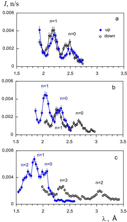
Fig. 13. The neutron microbeam intensity for spin up (closed symbols) and spin down (open symbols) vs. the neutron wavelength at the different applied magnetic field: (a) 300 Oe; (b) 1500 Oe; (c) 10.3 kOe. The grazing angle of the incident beam is  $0.133^\circ$ .
