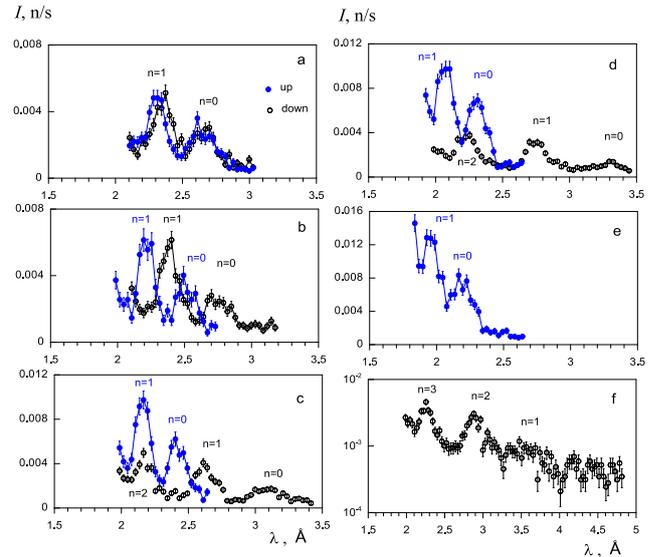
Fig. 14. The neutron microbeam intensity for spin up (closed symbols) and spin down (open symbols) vs. the neutron wavelength at the different applied magnetic field: (a) 600 Oe; (b) 1114 Oe; (c) 3030 Oe; (d) 5039 Oe; (e) 7001 Oe, spin up; (f) 7001 Oe, spin down. The grazing angle of the incident beam is  $0.145^\circ$ .
