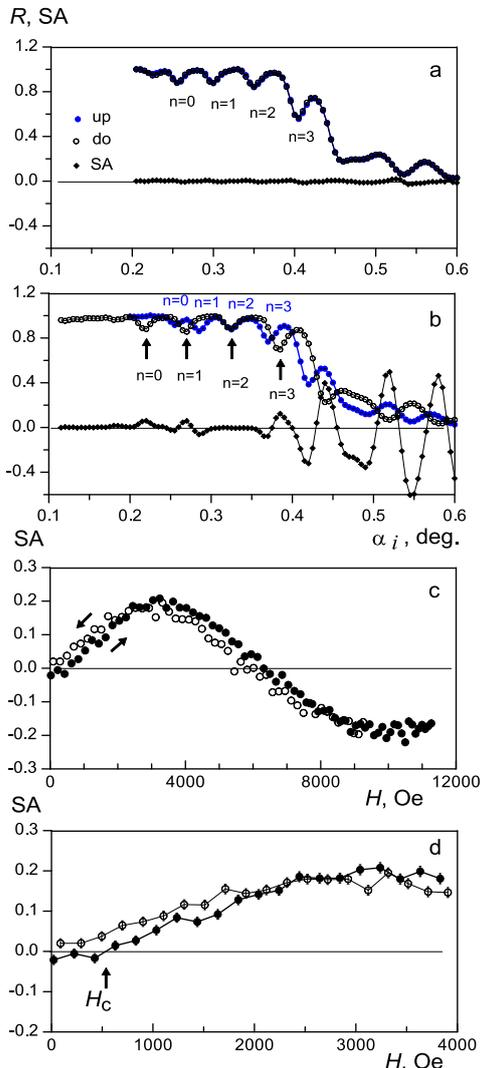
Fig. 5. Specular reflectivity  $R$  for spin down (open circles) and up (closed circles) and spin-asymmetry  $SA$  (rhombi) vs. the grazing angle of the incident beam for the applied magnetic field 386 Oe (a) and 4618 Oe (b). Spin-asymmetry at the grazing angle of the incident beam  $0.415^\circ$  vs. the applied increasing (closed symbols) and decreasing (open circles) magnetic field plotted in total interval (c) and in zoomed scale (d).
