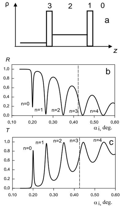
Fig. 2. Fabry-Perot interferometer: (a) SLD; (b) reflectivity; (c) transmission coefficient.
