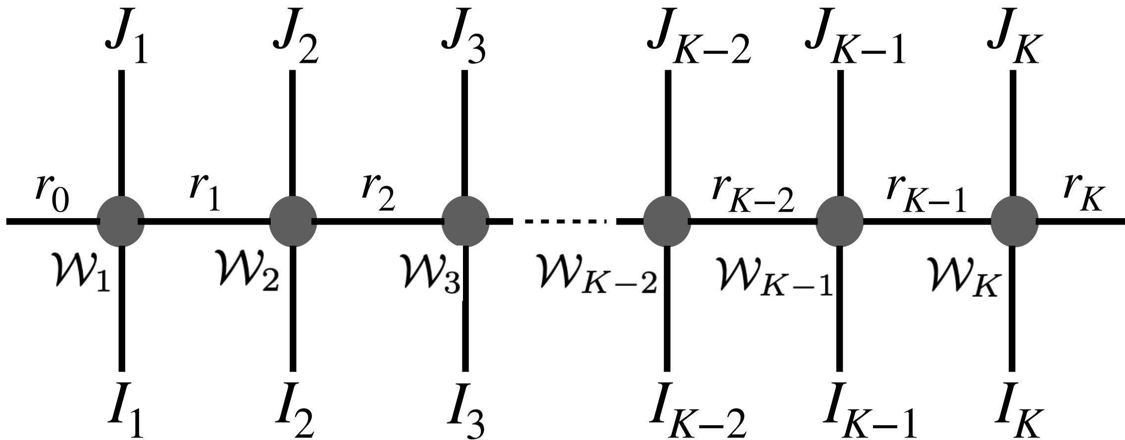
(a) Tensor-Train Network: given a set of TT-ranks  $\{r_1, r_2, \dots, r_K\}$ , a circle represents a core tensor and each line is related to a dimension.
