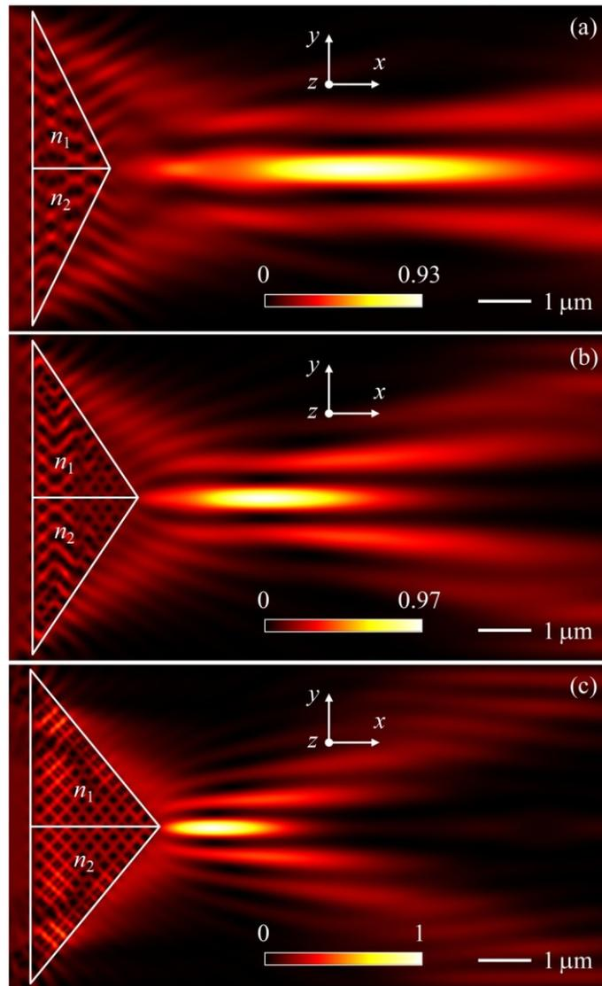
**Figure 2.** Normalized intensity distributions of the photonic nanojets formed by conventional triangular micro-prisms at (a)  $h = 1.5 \mu\text{m}$ , (b)  $h = 2 \mu\text{m}$ , and (c)  $h = 2.5 \mu\text{m}$ . The refractive index of triangular micro-prisms is  $n_1 = n_2 = 1.5$ .
