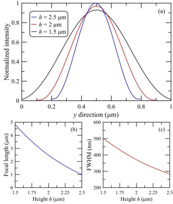
**Figure 3.** (a) Normalized intensity profiles of the photonic nanojets along  $y$  direction for conventional triangular micro-prisms. (b) Focal length and (c) FWHM as a function of the height  $h$  of the triangular micro-prisms.
