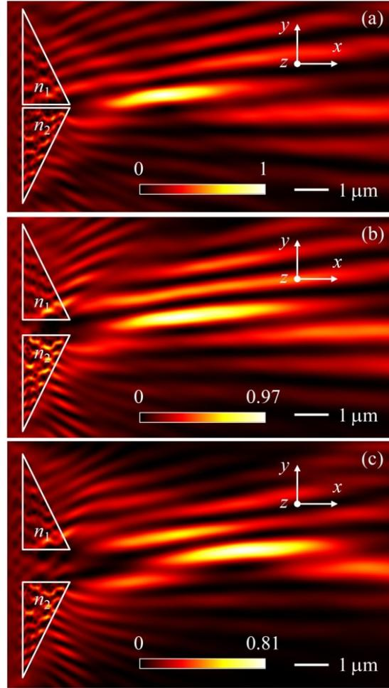
**Figure 6.** Normalized intensity distributions of the photonic hooks formed by triangular Janus micro-prisms at (a)  $d = 100$  nm, (b)  $d = 500$  nm, and (c)  $d = 1000$  nm. The refractive indices of triangular Janus micro-prisms are  $n_1 = 1.5$  and  $n_2 = 1.88$ .
