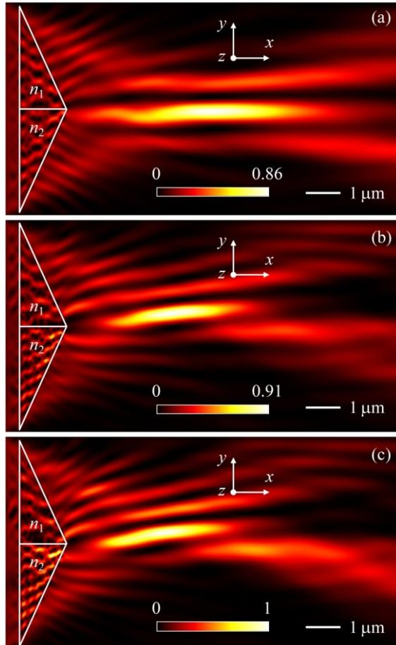
**Figure 4.** Normalized intensity distributions of the photonic hooks formed by triangular Janus micro-prisms at  $n_1 = 1.5$ , (a)  $n_2 = 1.58$ , (b)  $n_2 = 1.88$ , and (c)  $n_2 = 1.95$ . The height and width of triangular Janus micro-prisms are  $h = 1.5 \mu\text{m}$  and  $w = 3 \mu\text{m}$ .
