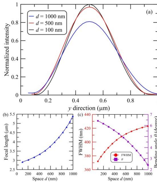
**Figure 7.** (a) Normalized intensity profiles of the photonic hooks along  $y$  direction for triangular Janus micro-prisms at different spaces  $d$ . (b) Focal length, (c) FWHM and bending angle as a function of the space  $d$  of the triangular micro-prisms.
