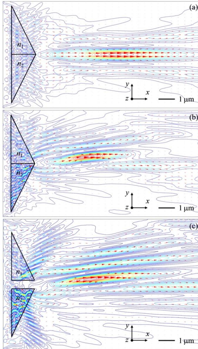
**Figure 8.** Poynting vectors and energy flow streamlines for triangular Janus micro-prisms at (a)  $n_1 = n_2 = 1.5$ , (b)  $n_1 = 1.5$ ,  $n_2 = 1.88$ , and (c)  $n_1 = 1.5$ ,  $n_2 = 1.88$ ,  $d = 500$  nm. The height and width of triangular Janus micro-prisms are  $h = 1.5$   $\mu\text{m}$  and  $w = 3$   $\mu\text{m}$ .
