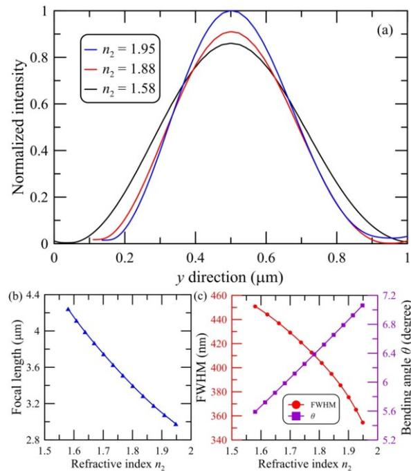
**Figure 5.** (a) Normalized intensity profiles of the photonic hooks along  $y$  direction for triangular Janus micro-prisms at different refractive index  $n_2$ . (b) Focal length, (c) FWHM and bending angle as a function of the refractive index  $n_2$  of the triangular micro-prisms
