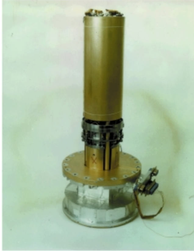
Figure 7. Existing XRS ADR Hardware will be used and designs copied to reduce cost.
