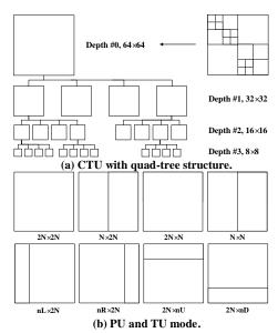
Fig. 1. Quadtree structure-based CTU/CU/PU Partitioning in HEVC.
