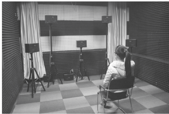
Figure 7 Subjective test setup. Subjective test environment and configuration.
