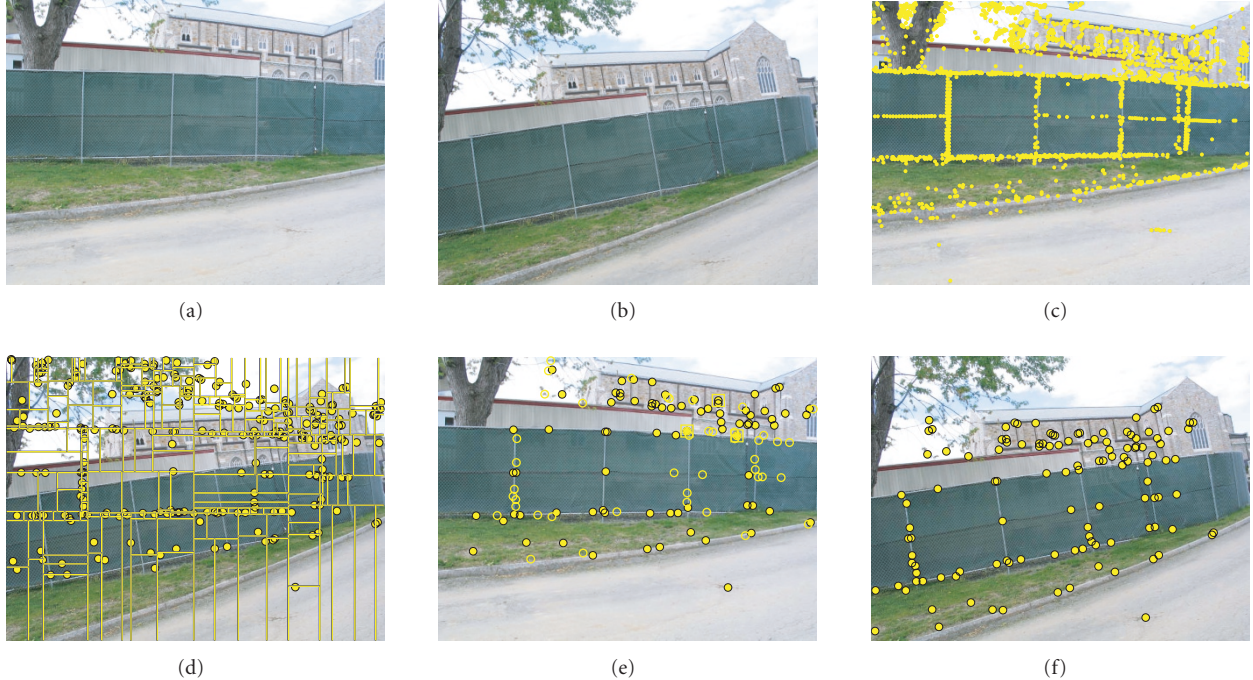
FIGURE 3: Example results of image matching from a pair of images. (a) Image 1. (b) Image 2. (c) The 1976 detected features in image 1. (d) The k-d tree and corresponding 256-feature digest in image 1. (e) The dots indicate 78 features in image 1 detected as correspondences in image 2, using the minimal Euclidean distance between SIFT descriptors and the ratio criterion with a threshold of 0.6. The 3 squares indicate outlier features that were rejected. The circles indicate 45 new correspondences that were grown based on the epipolar geometry, for a total of 120 correspondences. (f) The positions of the 120 corresponding features in image 2.
