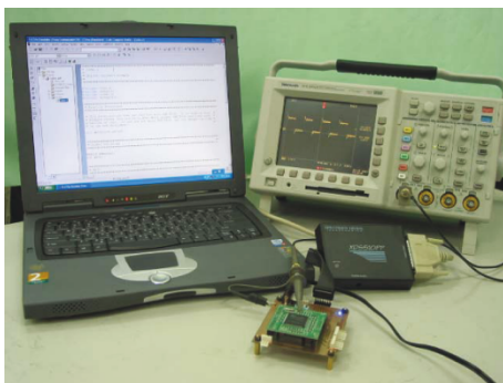
FIGURE 3: Laboratory workstation based on the self-developed DSP platform, which also shows PC, JTAG emulator and oscilloscope.
