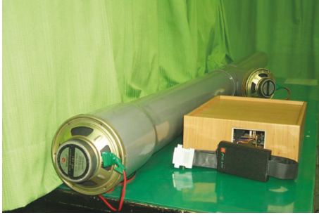
FIGURE 4: ANC laboratory workstation, which shows the self-developed DSP platform with JTAG emulator, a duct, and two loudspeakers.
