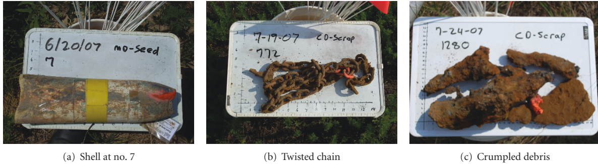
FIGURE 5: (a) Unexploded shell from Cell no. 7, and (b), (c) the two false alarms obtained by the SVM classifier using k and R as discriminators.
