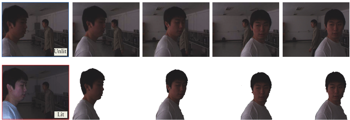
FIGURE 8: Segmentation of the “Moving Object and Background” sequence by the proposed algorithm I. The leftmost column shows a pair of unlit and lit frames, while the other columns show a series of unlit frames and their segmentation results.
