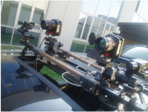
Figure 10 The tetra-vision far-infrared and daylight acquisition system installed on board of the test vehicle.
