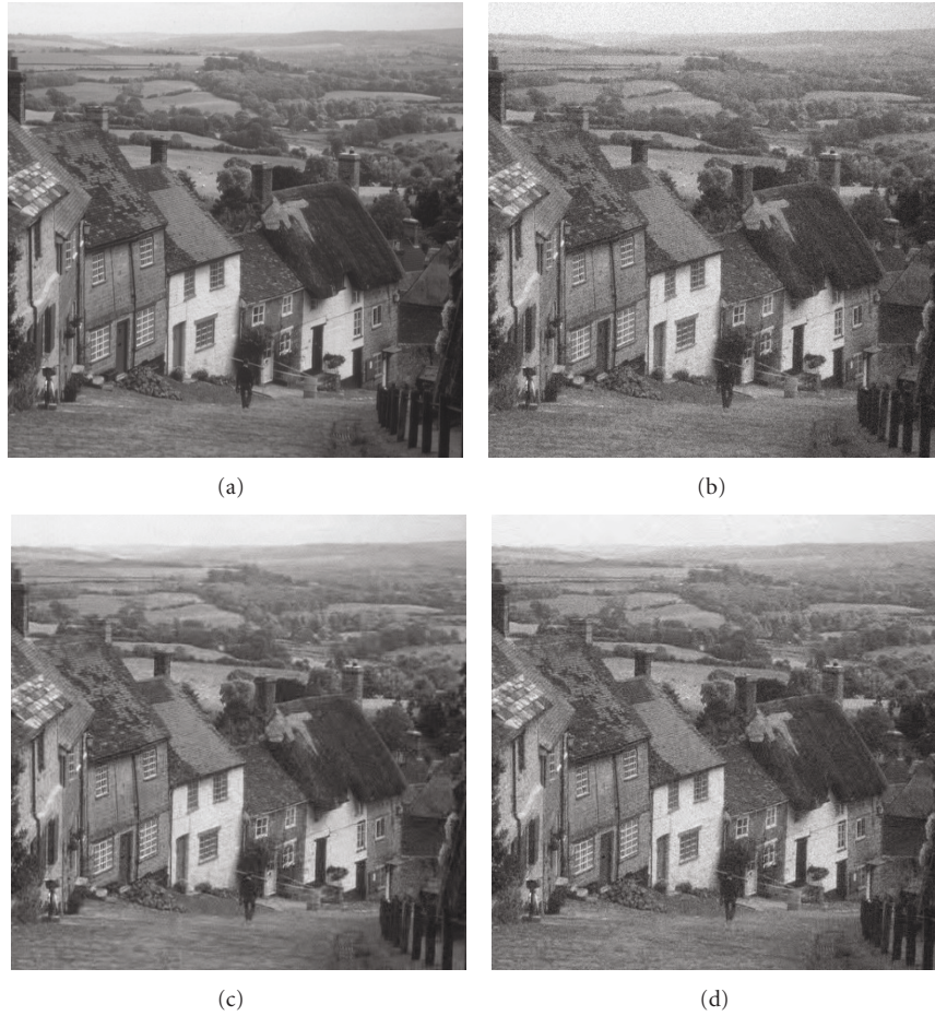
FIGURE 8: Image Goldhill: (a) noise-free, (b) noisy, \sigma^2 = 100 , (c) compressed by ADCTC, b = 3.5 , (d) compressed by AGU b = 3.5 .
