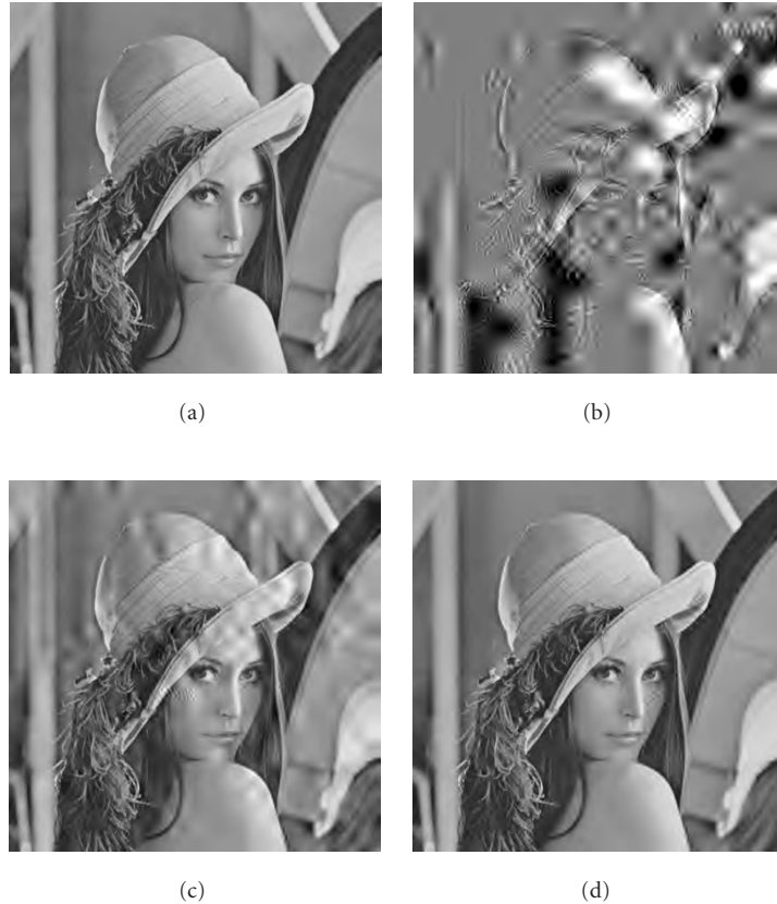
FIGURE 11: Performance of sequential decoding with JPEG-2000 coded images (courtesy of [24]). (a) JPEG-2000 coded; PSNR = 37.41 dB; no channel error. (b) JPEG-2000 coded; AWGN channel ( E_b/N_0 = 5 dB); PSNR = 16.43 dB. (c) JPEG-2000 coded with sequential decoding; AWGN channel ( E_b/N_0 = 5 dB); W = 10 ; PSNR = 25.15 dB. (d) JPEG-2000 with sequential decoding; AWGN channel ( E_b/N_0 = 5 dB); W = 20 ; PSNR = 31.91 dB.
