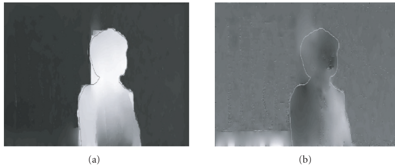
FIGURE 10: Boundaries of the manually segmented object superimposed to (a) the horizontal component of the optic flow and (b) the vertical component of the optic flow.
