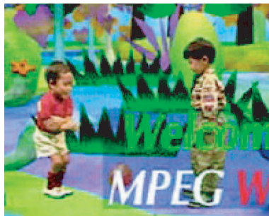
(b) One frame decoded by 14-bit FP 1-bit sign + 5-bit exp + 8-bit fraction.
