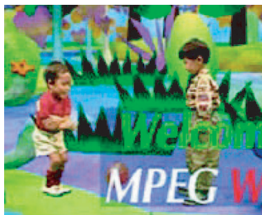
(a) One frame decoded by 32-bit FP 1-bit sign + 8-bit exp + 23-bit fraction.
