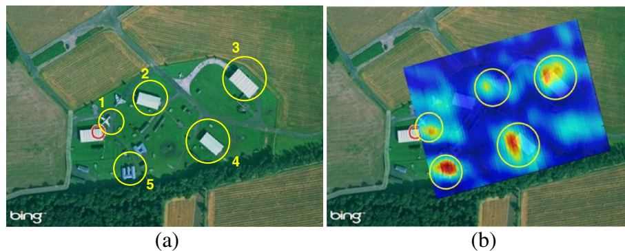
Figure 18 Imaging with Galileo and an airborne receiver: (a) Satellite photograph of imaging area, (b) experimental radar image super-imposed on imaging scene.
