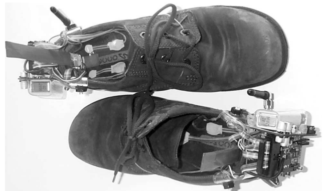
Fig. 3. GaitShoe hardware mounted on shoes.
