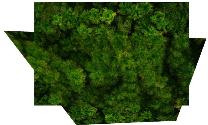
Figure 7: Deformation during mosaicking produced by the wrong estimation through RANSAC for two images with low overlap.
