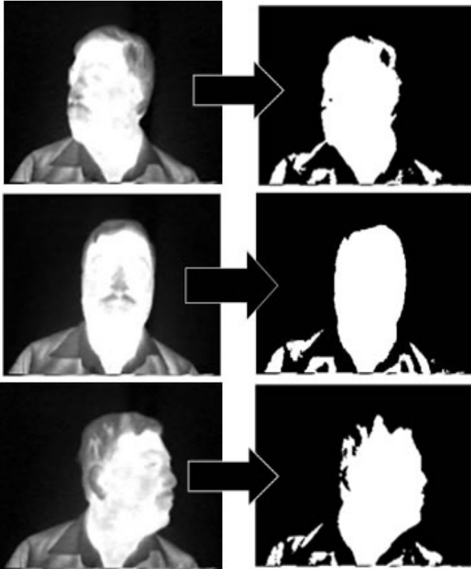
Figure10: Image from the Terravic Facial Infrared Database, before and after binarization.
