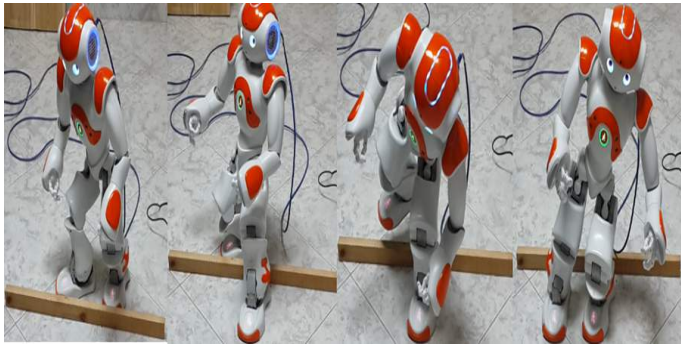
Figure 12: NAO steps over a 3.5 cm height and 2 cm depth wooden obstacle using planned whole body movement
