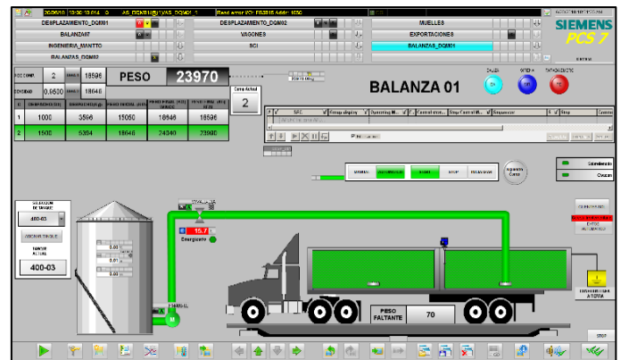
Figure 14: Electrical valve restricted to 15%, for a lack weight less than 70 kg. - compartment 2
