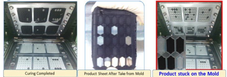
Figure 3: Defect auto Deflash
