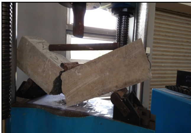
Figure 6: Flexural strength test
