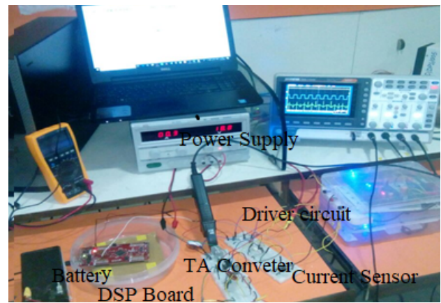
Figure 12: Picture of the hardware setup of the proposed TA Converter with DSP and PC interface.
