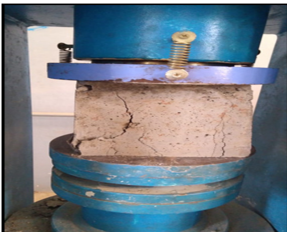
Figure 2: Compressive strength test
