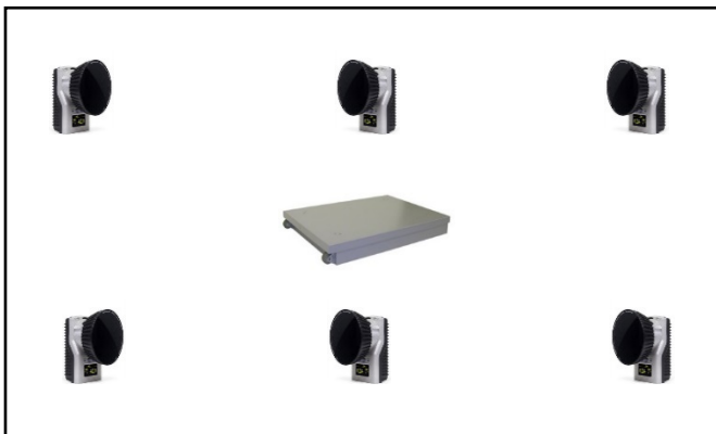
Figure 2: The field set-up of infrared cameras relative to the force platform
