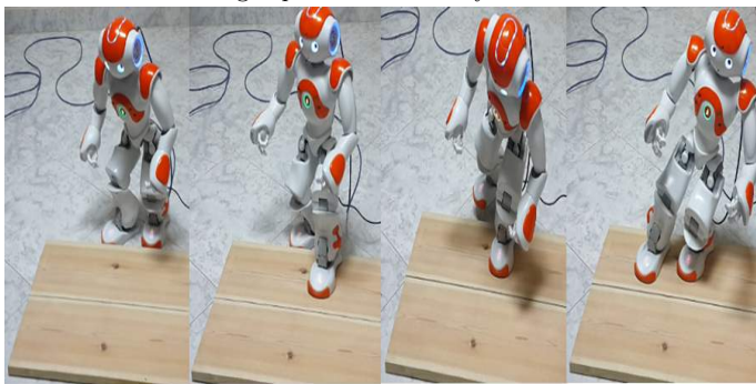
Figure 14: NAO step 2 cm high and 40 cm deep on a wooden obstacle using the expected whole body movement
