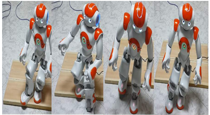
Figure 15: NAO descending from a 2 cm height and 40 cm depth wooden obstacle using the expected whole body movement
