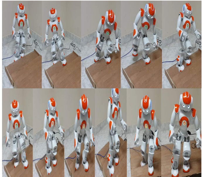
Figure 16: NAO ascending 4 cm high and 20 cm deep stairs using the expected entire body movement
