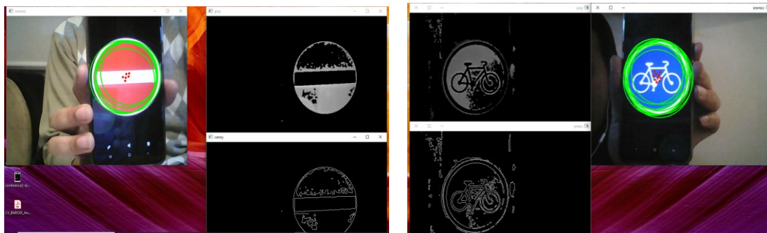
(a) Red signs (b) Blue signs Figure 3: Traffic Signs detection manual thresholding [5]
