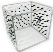
Figure 2: An acoustic camera capable of underwater operation [34]
