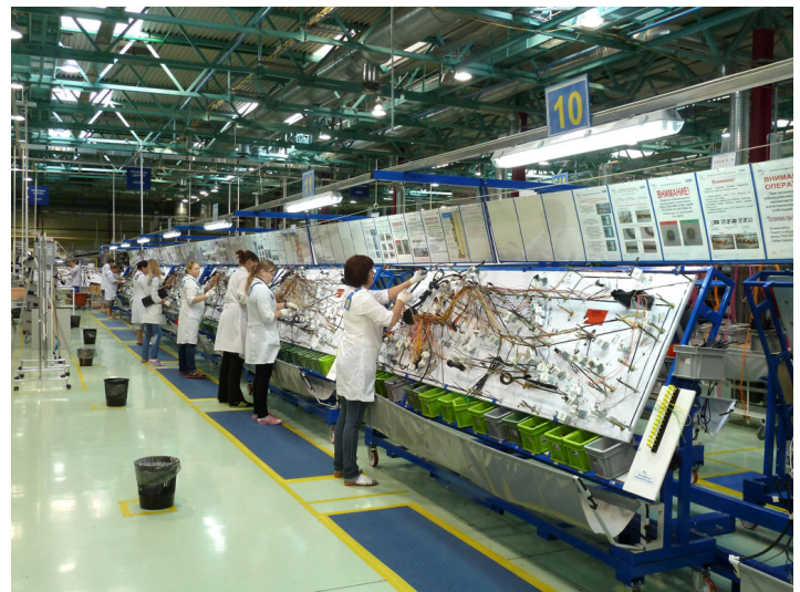
Figure 6: The photo shows a wire harness production facility where workers assemble prefabricated wires into a wire harness. Photo: OWC.
