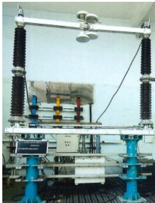
Figure 7: Switching Capability Type Test Set-Up of a 245kV Center Break Disconnector with a Passive Add-On Finger Solution
