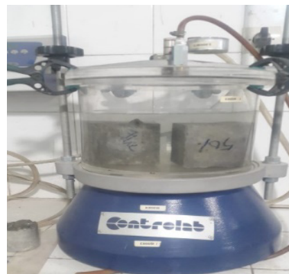
Figure 3: the test pieces placed in the vacuum apparatus for 24 hours
