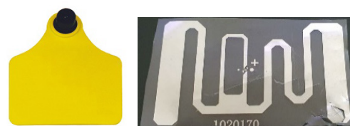
Figure 7: Ear tag and embedded UHF antenna used for identification
