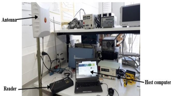
Figure 10: The Read range measurement setup
