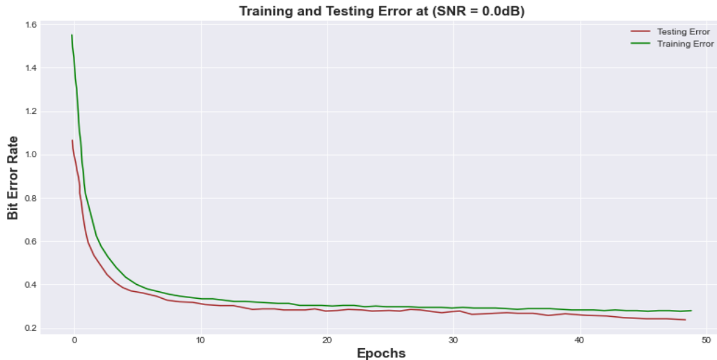
Figure 15: Bit Error Rate vs Training Epochs for FCNN Autoencoder at (SNR= 0.0 dB) channel.
