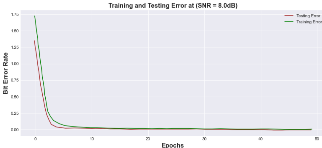
Figure 16: Bit Error Rate vs Training Epochs for FCNN Autoencoder at (SNR= 8.0 dB) channel
