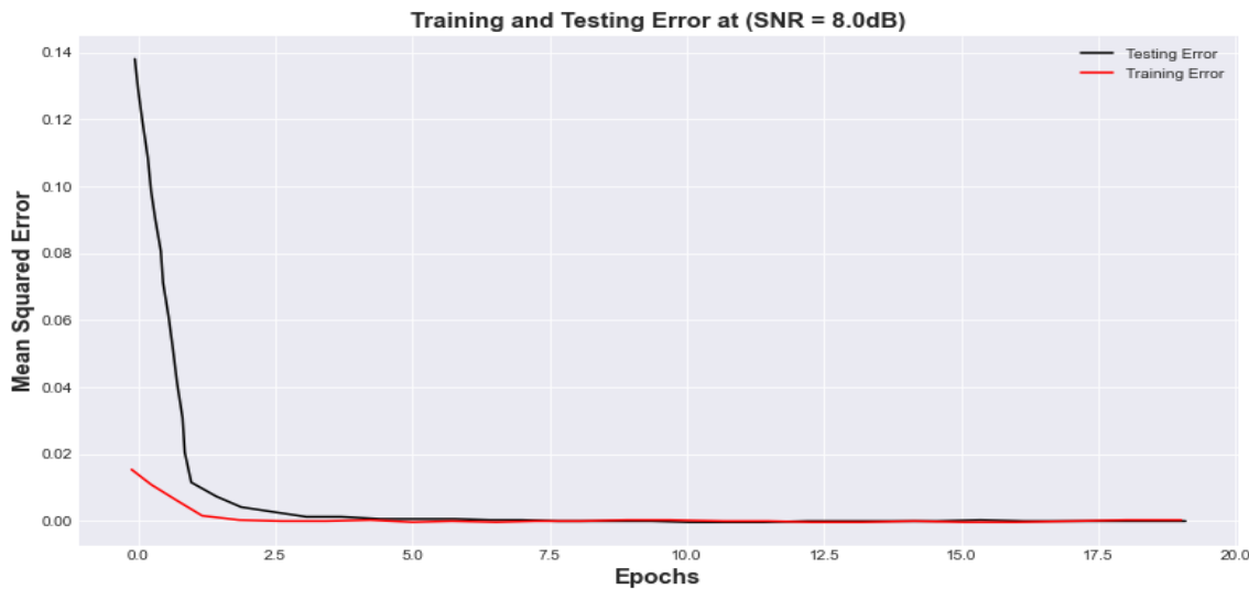
Figure 18: Mean Squared Error vs Training Epochs for BLSTM Autoencoder at (SNR= 8.0 dB) channel
