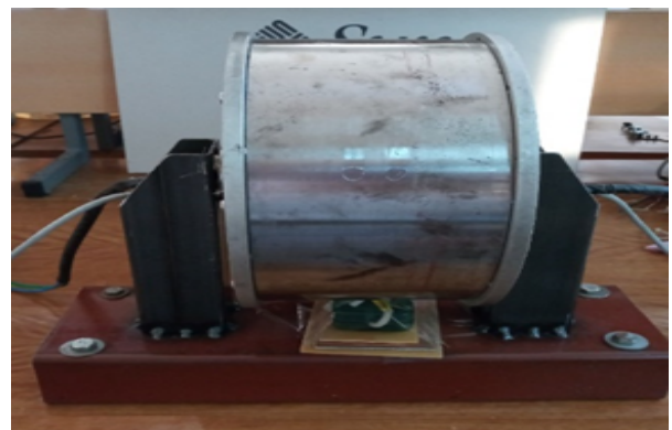
Figure 14: Experimental Setup of Hub BLDC Motor.
