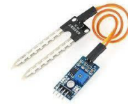
Figure 3: (A) The soil moisture sensor,
