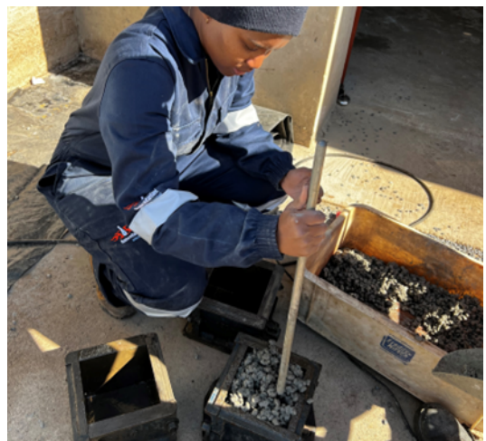
Figure 12: Compacting with a rod.
