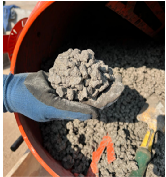
Figure 10: Ball Method (PC consistency check)
