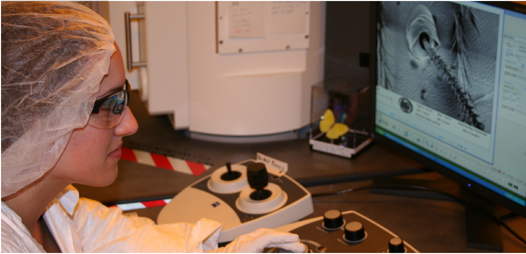
A graduate of the Nanofabrication Manufacturing Technology capstone program at Penn State University demonstrates how to image a biological sample, in this case a spider, using a field emission scanning electron microscope. Students from around the country use remote access technologies for real-time interactions with people and equipment in the nanotechnology lab at University Park, Pennsylvania.
