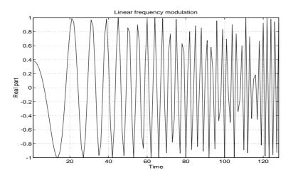
Figure 1.1: Linear frequency modulation (chirp)
