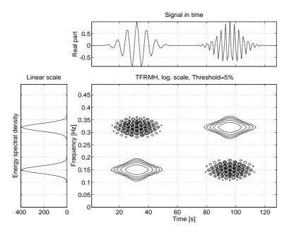
Figure 4.14: Margenau-Hill distribution of 2 atoms : the position of the interferences is quite different from the one obtained with the WVD
