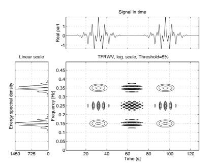
Figure 4.4: WVD of 4 gaussian atoms : many interferences are present
