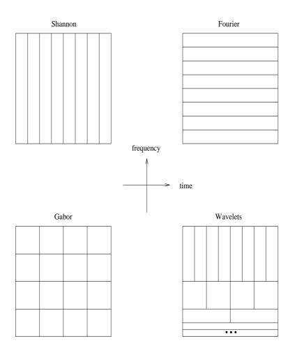
Figure 3.14: Sampling of the time-frequency plane. Different forms of sampling: Shannon, Fourier, Gabor, Wavelet
