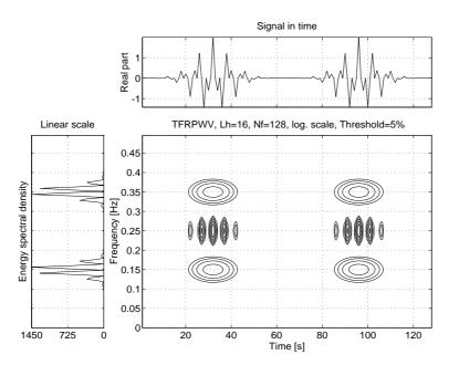
Figure 4.5: The frequency-smoothing operated by the pseudo-WVD attenuates the interferences oscillating perpendicularly to the frequency axis
