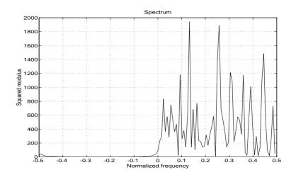
Figure 1.5: Energy spectrum of the noisy chirp
