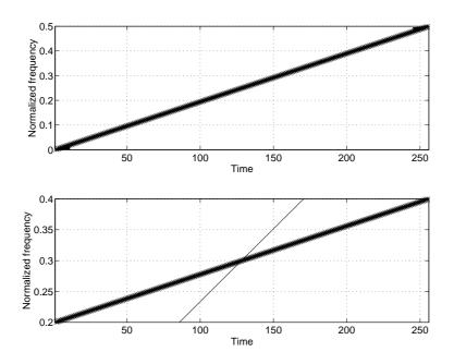
Figure 2.5: Estimation of the instantaneous frequency (stars) and group delay (line) of two different chirps with different amplitude modulations. The first plot corresponds to a large  $T \times B$  product while the second corresponds to a small one
