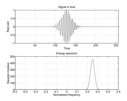
Figure 2.1: Linear chirp with a gaussian amplitude modulation
