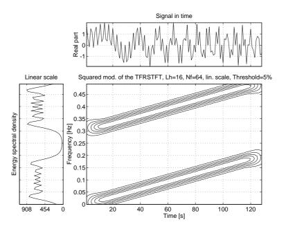
Figure 2.11: Squared modulus of the short-time Fourier transform of the previous multi-component non-stationary signal
