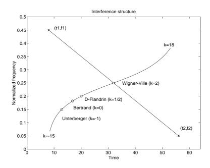
Figure 4.26: Locus of the interferences between 2 points for the affine Wigner distributions (parameterized by k). For k = 2, which corresponds to the Wigner-Ville distribution, we obtain the geometric mid-point
