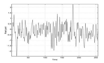
Figure 2.9: Gaussian transient signal (sig1) embedded in a  $-10\,\mathrm{dB}$  colored gaussian noise
