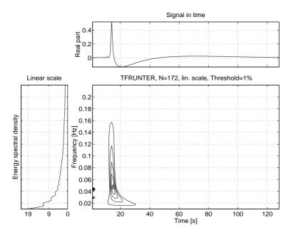
Figure 4.23: Active Unterberger distribution of a signal with a group delay in  $1/\nu^2$
