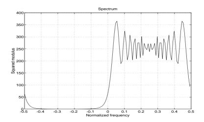
Figure 1.2: Energy spectrum of the chirp
