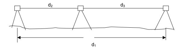
To carry out this test, three tripods are set up with tribrachs in a straight level line. Distances  $d_2$  and  $d_3$  should be integer multiples of 10 within say 0.05 m to eliminate any cyclic error affect, qv. Scale error will not affect this test. The prism and the EDM are both fitted with forced centring bases to fit into the tribrachs, and can be interchanged on the tripod/tribrachs with no centring error. Thus any discrepancy in the measurements is purely zero error of the system.
