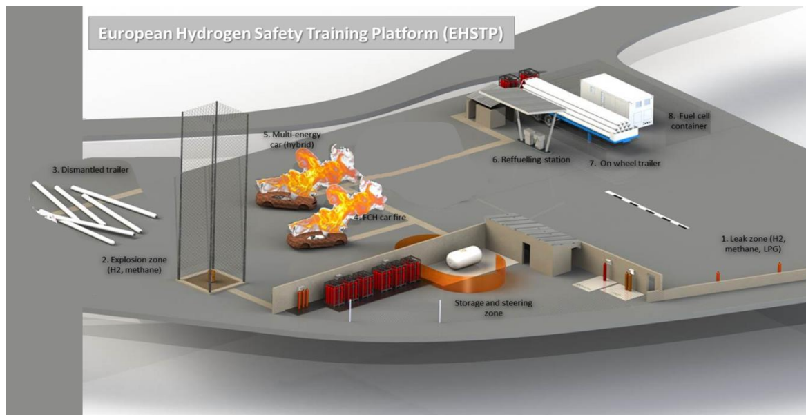
Figure 9.1: European Hydrogen Safety Training Platform (EHSTP). 2500 m 2 ; fuel comparison using hydrogen (700, 350 and 200 bar), CNG (200 bar) and LPG (20 bar)
