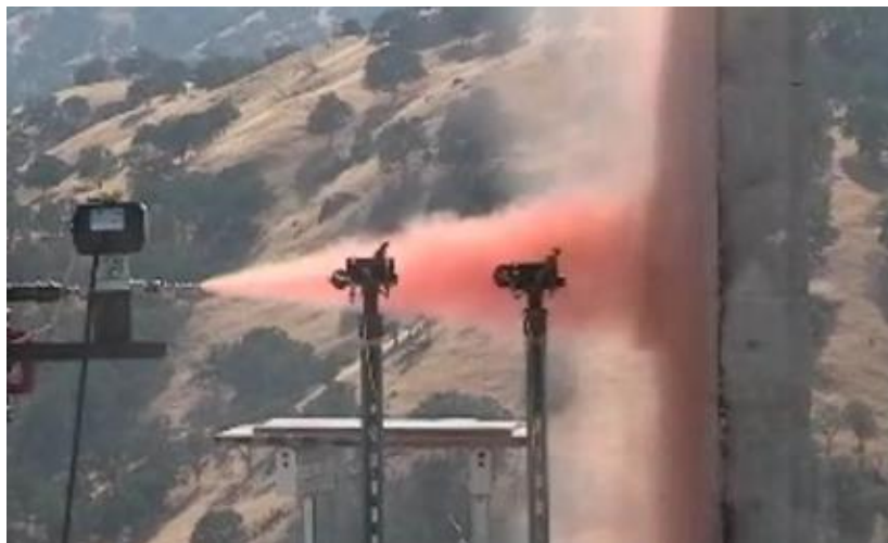
Fig. 4.9: On the left is an example of spontaneous ignition exiting a shock tube [23], ignition occurred 100% of the time – shock heating. On the right is a delayed spontaneous ignition from a choked flow exit the ignition point is in subsonic flow ignition occurred 100% of the time (shock heating is not the source) [24].
