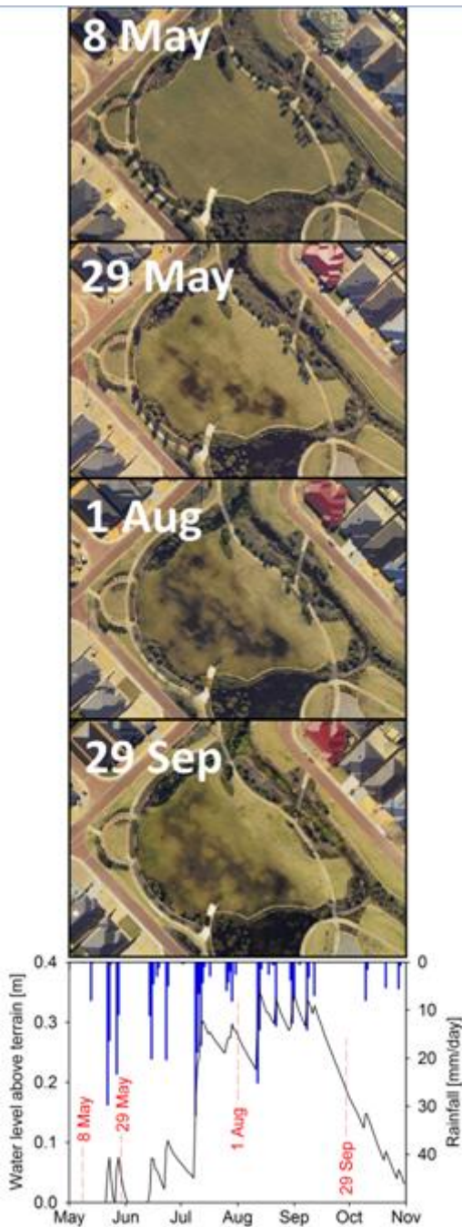
Figure 11. Aerial photos together with the simulated water level above terrain at the Auckland Parade detention basin during the year 2010. The aerial photos show water standing on the green area of the Auckland Parade.
