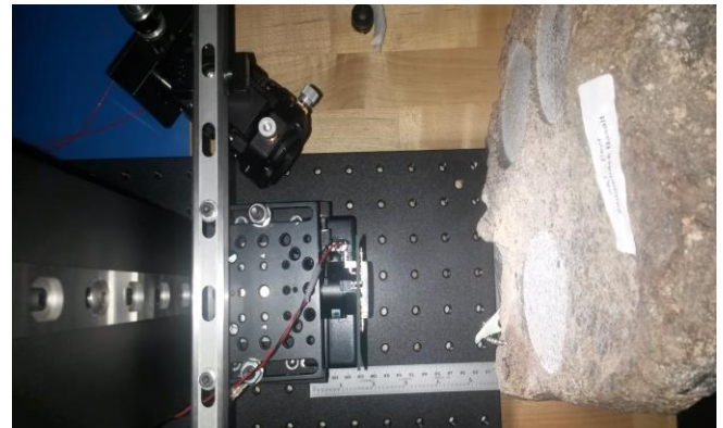
Figure 19: The structured light system consisting of the CCD sensor, laser source (black box at angle at top of image). In this specific image, the system is measuring the distance to an abraded Saddleback Basalt sample.
