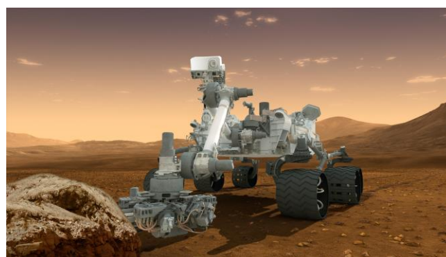
Figure 1: Artist conception of the rover taking a measurement with a turret mounted instrument on the Mars Rover Robotic Arm. (Credit NASA/JPL)
