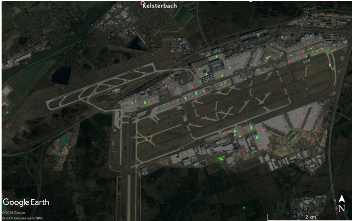
Fig. 2. Part of Fig. 1 bottom row right overlaid in Google Earth. We see significant changes based on the Wishart change detector combined with direction of change based on the Loewner order occurring where aircraft at gates, on aprons, taxiways and runways, cars in parking lots and on the motorways, and ships on the River Main come and go. Overlaid colors are interpreted as: present at time point one and not at time point two (red), present at time point two and not at time point one (green), significant change but the nature of the change is such that the Loewner order cannot decide the direction (yellow).
