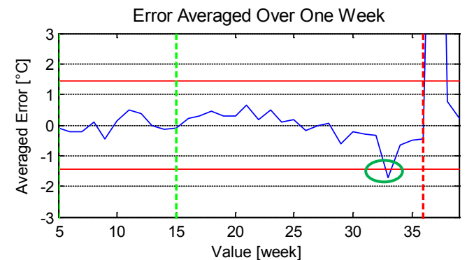
Figure 26: Averaged prediction error of the FSRC neural network model including the training period
