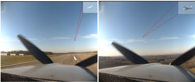
Fig. 1. Visualization of the detected aircraft bounding boxes from the data onboard a general aviation aircraft. At long ranges, the SnR is really poor, and our algorithms are trained to detect aircraft even in low SnR situations.
